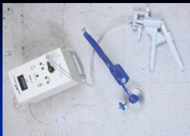
Poroscope (Figg Air Permeability Test)
