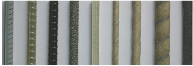
Fig 8. Examples of glass and carbon FRP bars and rods
