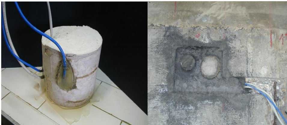
Fig. 3. Example of the instrumentation of an existing RC structure damaged by reinforcement corrosion and submitted to repair works.
