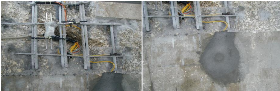
Fig. 22. Detailed aspects of the installation of sensors. In areas without concrete removal one cores instrumented with a resistivity sensor was fixed. A reference electrode was installed in the interfacial zone between area with complete removal of concrete cover and areas where the concrete was not removed
