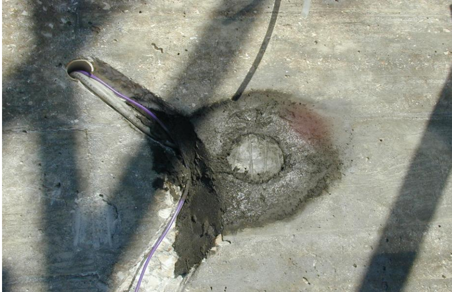
Fig. 21. Instrumentation of an area without removal of concrete cover.
