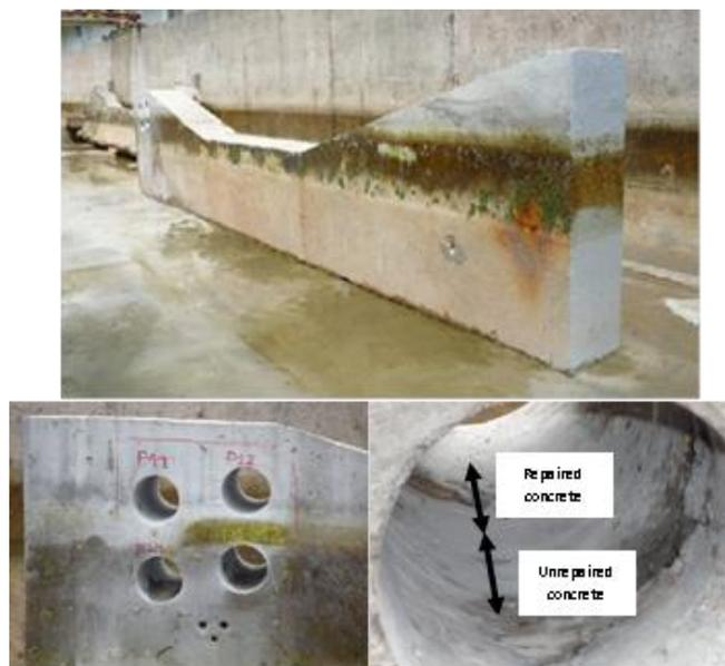
Figure 13 .Beams repaired in natural site
