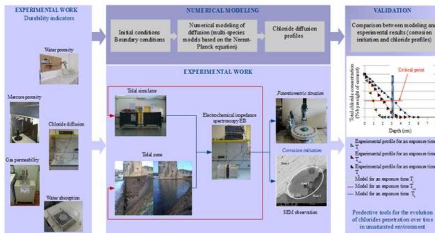
Fig.9. Experimental and numerical modelling methodologies
