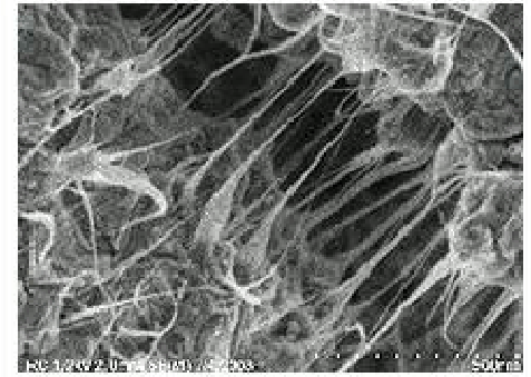
CARBON NANOTUBES FILLING THE CRACKS IN A CEMENTING COMPOSITE
