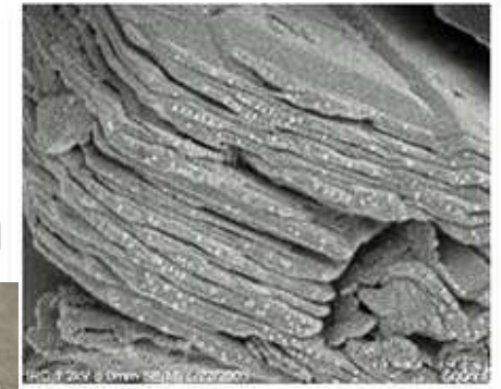
NANOLAYERS OF CALCIUM ALUMINATE
