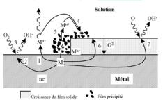
Fig. 4.1.2 Widespread comosion process involving phenomena of charge transfer, film formation and transport processes, from ASM Handbook (1987)).
