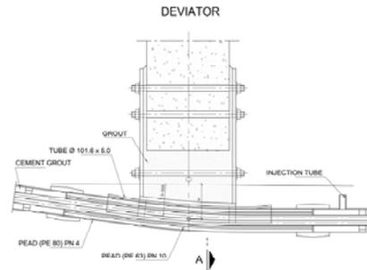
Fig. 7.10 - External prestressing of the approach viaducts and details
