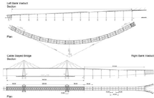
Fig. 7.1 - General view and dimensioning of the bridge
