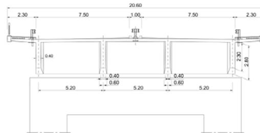
Fig. 7.3 - Transverse section of the approach viaduct
