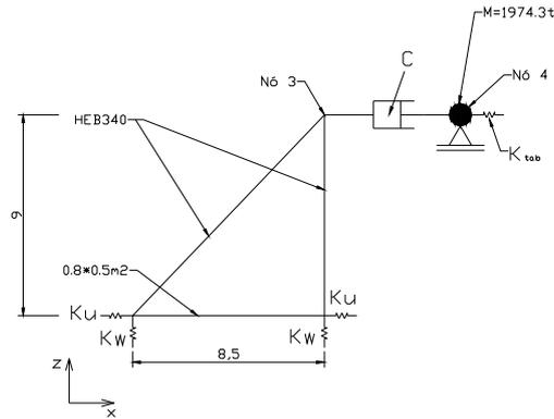
Fig. 5.5 - Structural model
