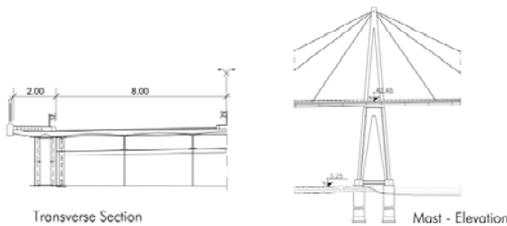
Fig. 7.2 - Dimensioning of the cable stayed bridge
