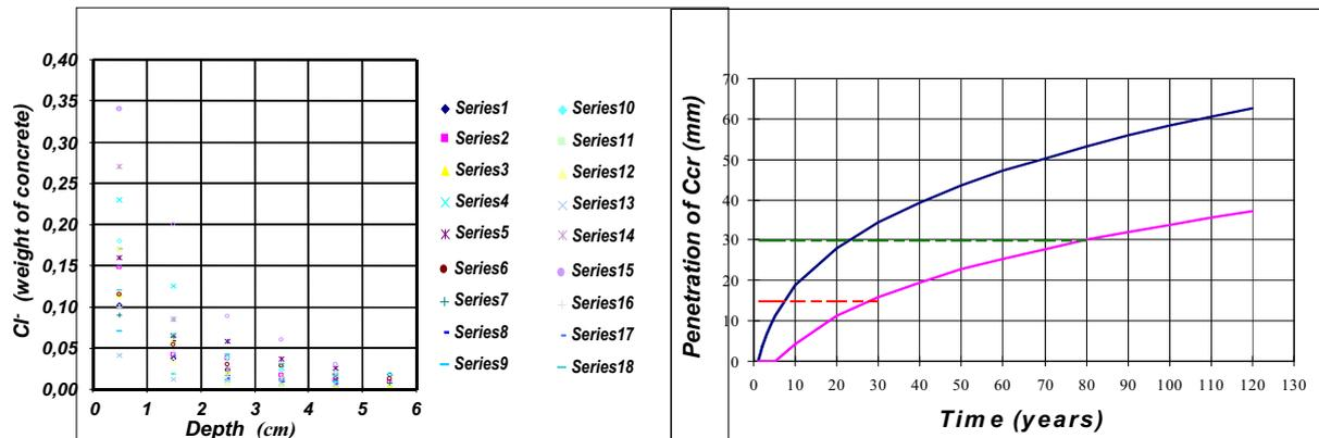
Fig. 6.4a - Chloride penetration near construction joints in the girders
