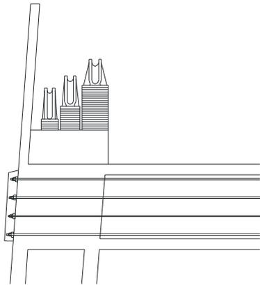
Fig. 7.8 - Strengthening of the transverse top beam of the towers
