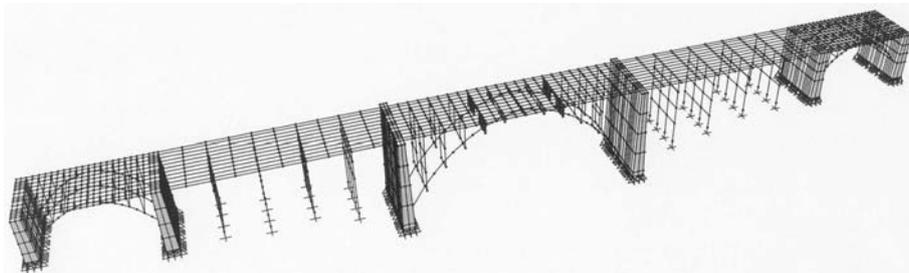
Fig.3.10. - Three Dimensional Model and Restraints
