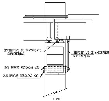
Fig. 7.9 - Replacing and strengthening the anchorage system of the deck to the transition piers
