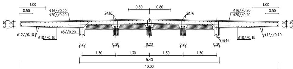
Fig.1.9 - Enlargement and strengthening of the slab
