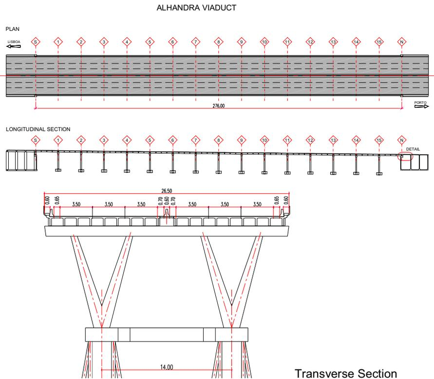
Fig. 5.1 - General dimensioning (dimensions in meters)
