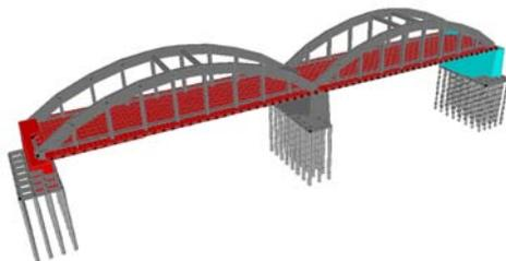
Fig 2.7 - Structural model of the bridge
