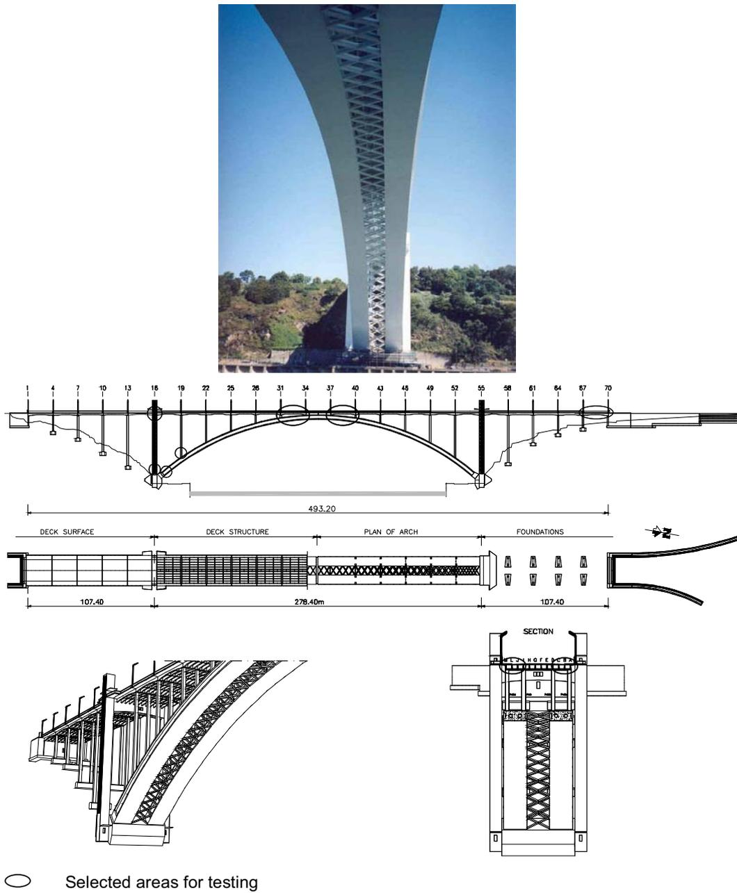
Fig 6.1 - Arrabida Bridge dimensioning and selected areas for testing
